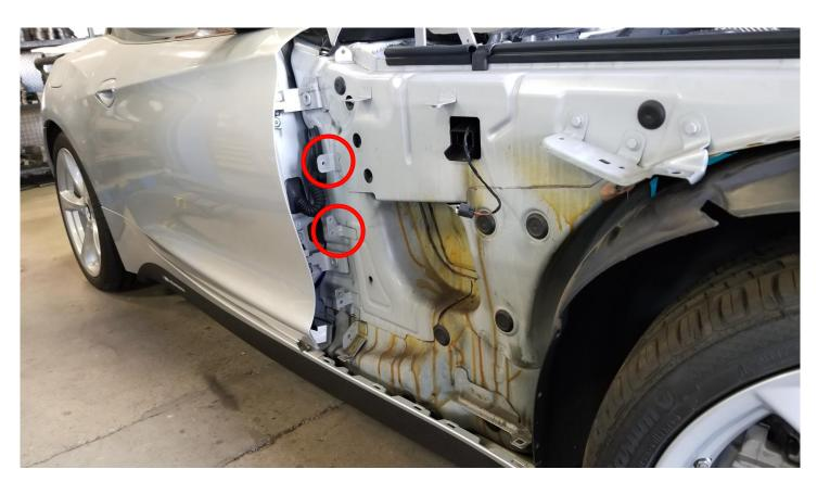
Before removing the factory door hinges, make sure to mark the factory location of the door.
