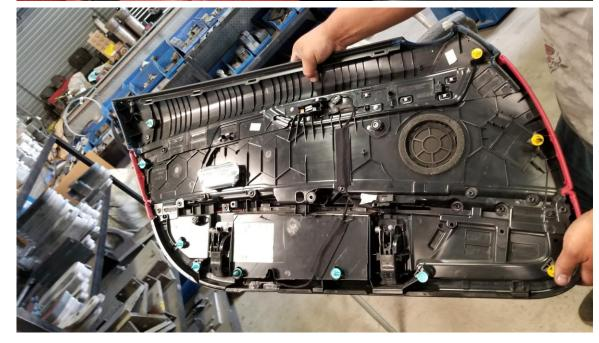
After removing the door panel pull back on the plastic over. Remove the speaker, this will allow you to remove the door catch. You will need to remove the censor at the top front of the door and elongate its wire.
