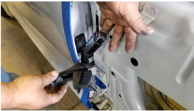
After carefully marking the factory location of the door, you will need to remove it.
