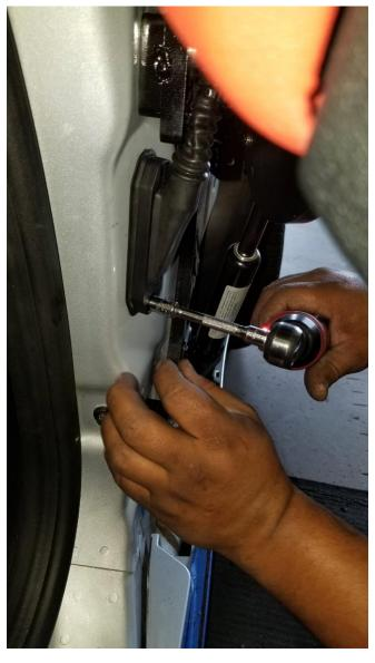
Once hinge is locked in place, break nut #1 then turn Allen set screw #2 on fig until it hits the block then open the door and continue to adjust until the door matches with the striker, open and close door making sure it closes like factory.
