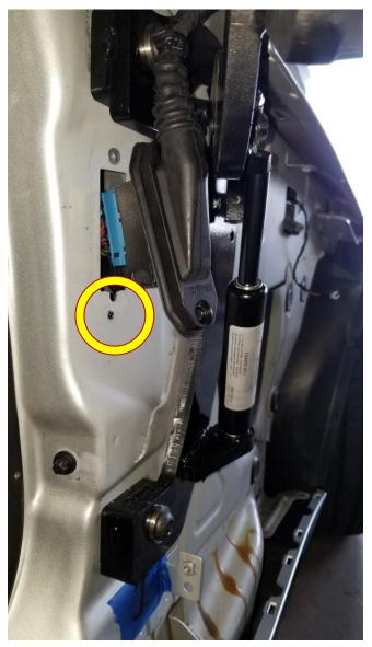
Secure the wire harness to the apron in the upside-down position.
