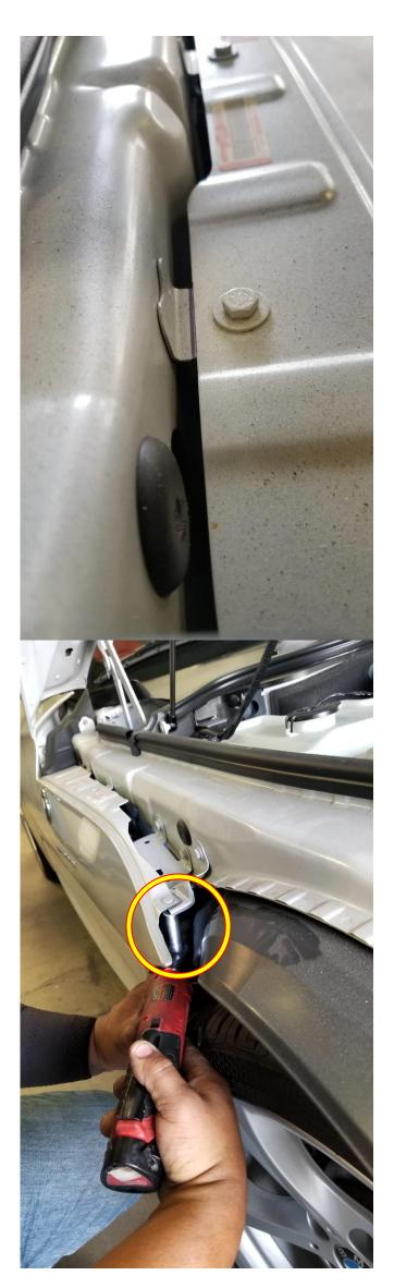
When removing the fender carefully remove the plug on the side marker and the remaining bolt form the top, pull on the fender to get access to the bolt inside the fender by the door.
